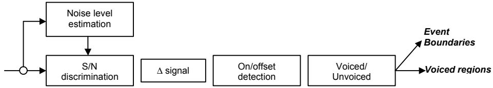
Figure 2. The pre-processing stage of the system developed. An audio signal given in input is segmented into musically meaningful events. Each event is characterized by its location in time (event boundaries) and by its voiced region.
